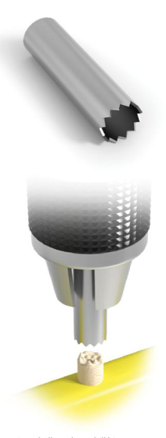
By using a hollowed-out drill bit, you can remove a broken dowel such as one used in the leading edge of the wing. First, find a piece of metal tube that can slide over the broken dowel. File cutting teeth in one end of the tube and then insert the other end in your drill. Use this to "core out" the broken stub. Use this same method to remove broken-off screws.
